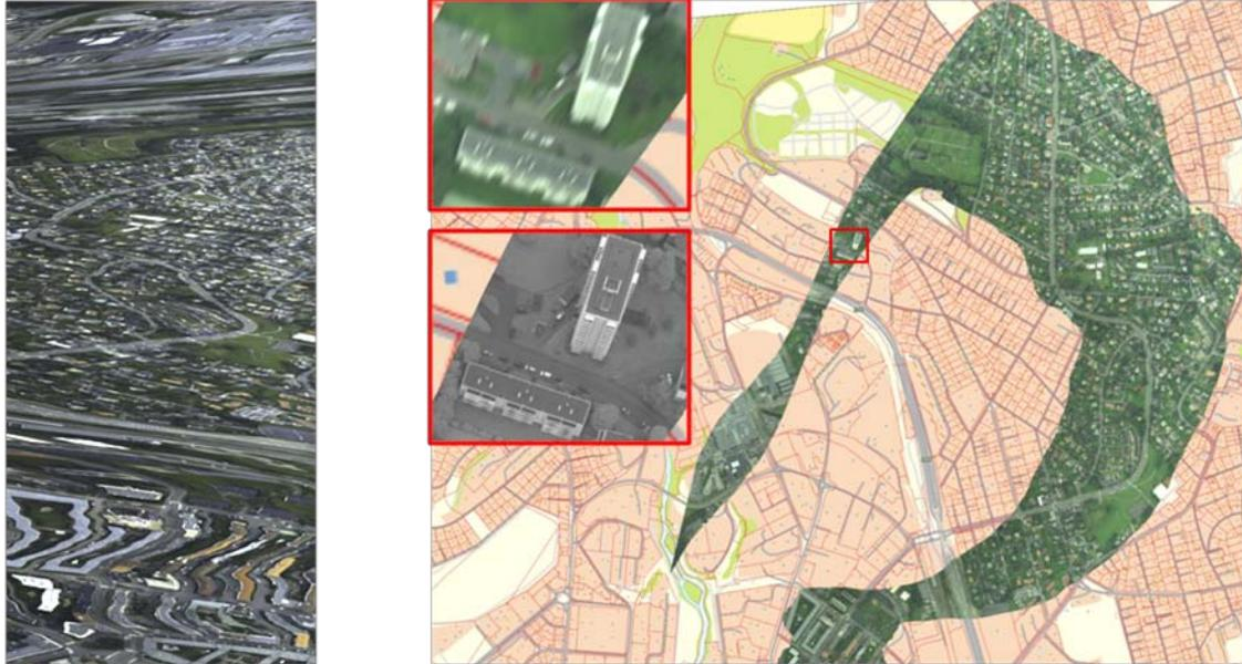
Figure 4. The leftmost image is an RGB representation of a raw HS image taken during a sharp left banking turn. To the right, the same image is shown rectified on top of a topographic map<sup>6</sup> in HyView. Zoom images from the HS and HR imagery have been added to illustrate the quality of the rectification.
