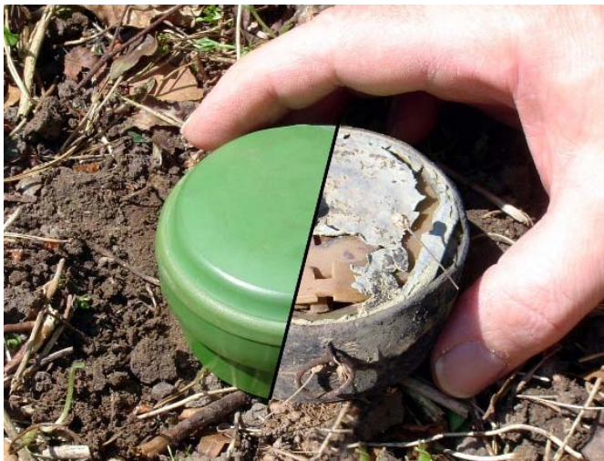
Figure 3.4 A manipulated picture showing the deterioration of a Type 72 mine. (photo Colin King)
