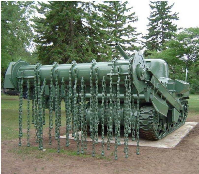
Figure 4.1 Flails for mine clearance put on a tank. Upon use, the drum will rotate with high speed.
