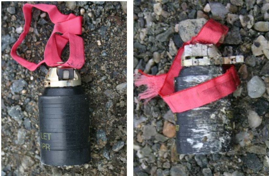
Figure 3.2 Bomblet DM1385 found in an unarmed state (left) and an armed state (right)
