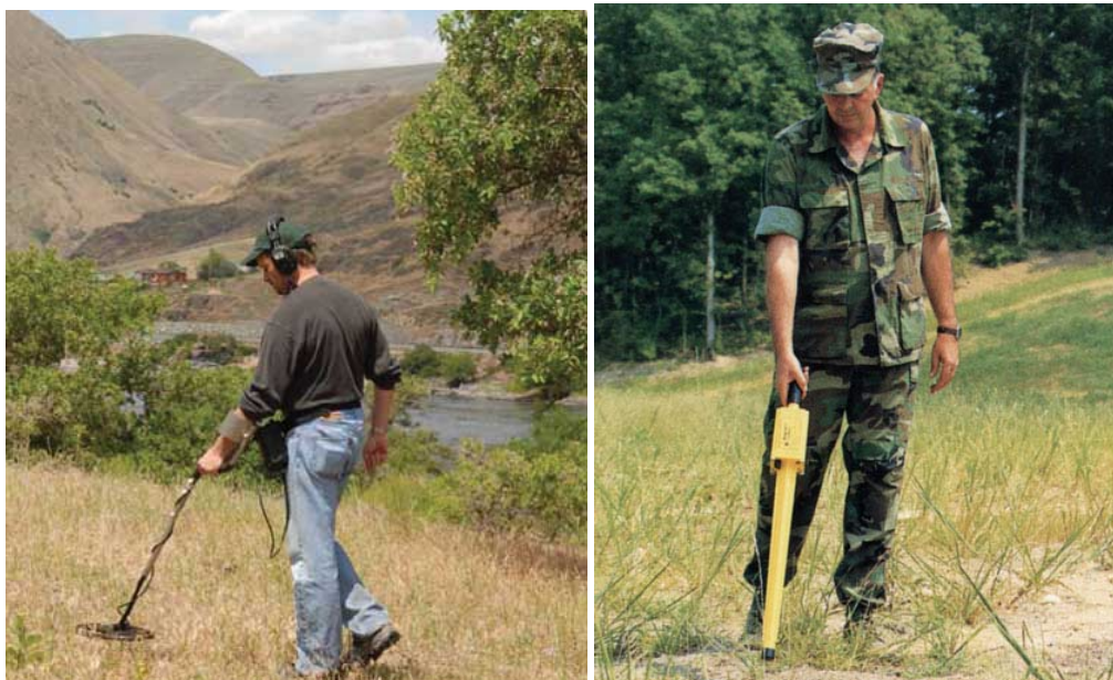
Figure 3.1 The metal detector (left) is based on detecting changes in the electric conductivity, while the magnetic detector (right) detects changes in the magnetic field.
