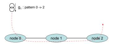
Figure 7.1 A chain of three nodes with one active traffic generator. The generator sends packets from end source 0 to end destination 2, and does not request use of ARQ.
