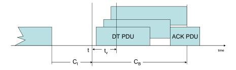
Figure 3.11 The contention phase and the transmission phase of a channel access cycle. The first node transmits at time instance t and a listening node detects a busy channel at  $t + t_v$ . The system uses immediate acknowledgment which means an ACK is returned without any delay and may collide with on ongoing data transmission (packets may have different lengths).
