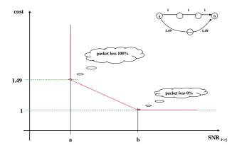
Figure 5.7 The radio links are assigned a cost factor according to the SNR-level. The demodulation threshold cost value is set to 1.49 to force the routing to select the two hops routing path instead of three hops at the upper right corner of the figure.
