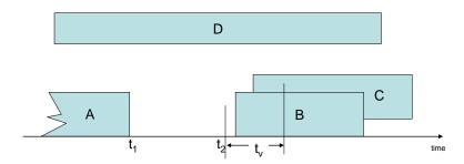
Figure 6.12 A packet transmission ends at  $t_1$  and all busy nodes within the neighbourhood that have a common understanding of an idle channel state start their MAC scheduling.
