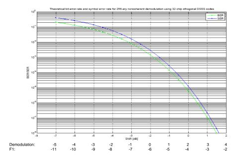
Figure A.1 SER versus SNR for demodulation (CRC16, LI and PHY payload) and F1.
