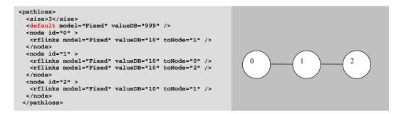
Figure 5.4 This example gives a chain of 3 nodes (since 999 dB pathloss stops all RF waves while 10 dB is a very low attenuation).
