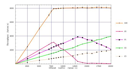
Figure 9.6 Throughput versus offered traffic. No confidence control is used for the plots showing throughput per priority. Radio version: 100kbps (simNov26a).
