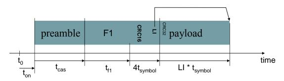
Figure 3.13 oTWLAN air frame format.
