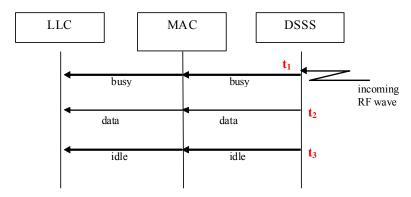
Figure 6.10 Sequence diagram for successful packet reception. Note the local control signals which are forwarded by the MAC module to the LLC module.
