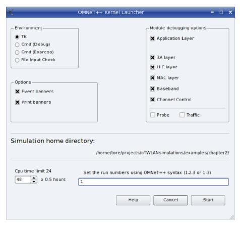
Figure 2.15 The simulator's kernel launcher (class GUI\_OmnetStartEditor).
