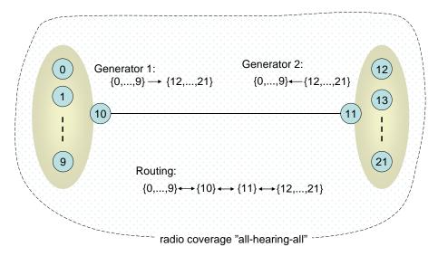
Figure 10.1 A fully-connected network containing 22 nodes where the traffic is forced to traverse 3-hops.
