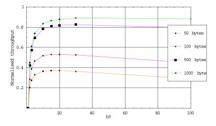
Figure 9.1 Normalised throughput as function of  $b_3$  in a network with 25 active nodes. The legend expresses the L7 payload size.
