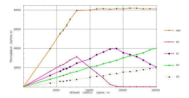
Figure 9.7 Throughput versus offered traffic. No confidence control is used for the plots showing throughput per priority. Radio version: 1Mbps (simNov26c).
