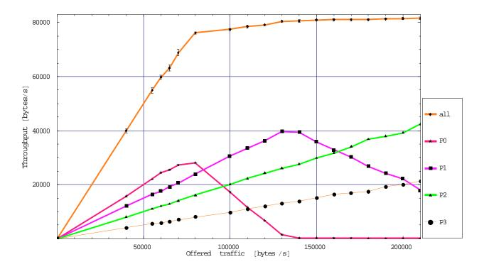
Figure 2.18 Network throughput versus offered traffic. The total throughput is presented as 90% confidence intervals while no confidence control is applied for the other plots (examples/chapter2).
