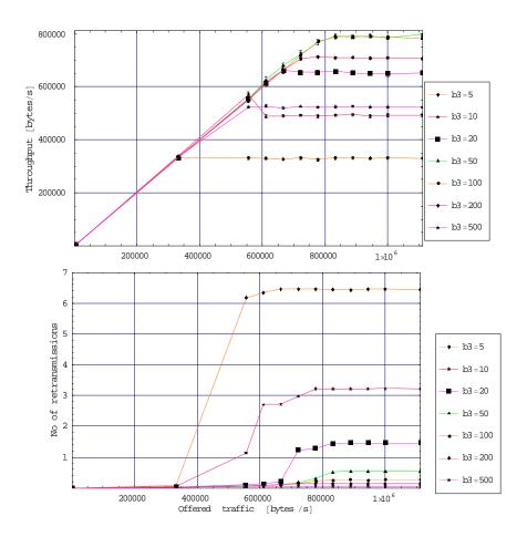
Figure 9.4 Throughput as 90% confidence intervals (top picture) for the 10Mbps radio version.
