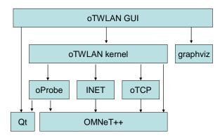
Figure 7.3 Software dependency graph. oTCP is an optional module.
