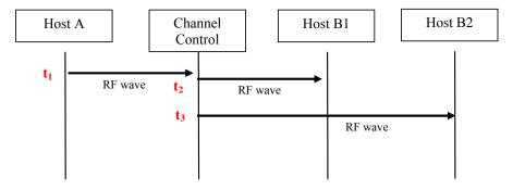
Sequence diagram for radio wave propagation when host A transmits. The MChannelControl distributes the wave to all hosts within the radio coverage area of host A.
