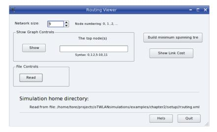
Figure 2.10 The "Routing Viewer"-widget (class GUI\_Routing).
