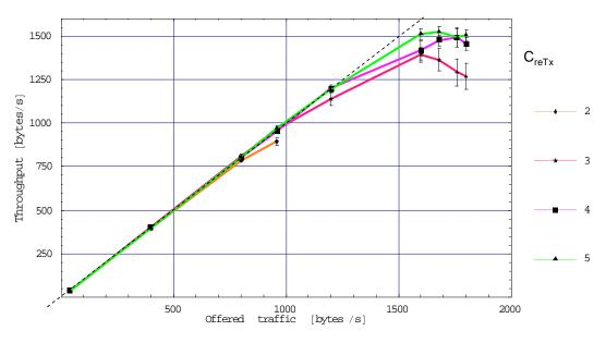
Figure 10.3 Case A3 throughput capacity for different multiplying constants  $C_{reTx}$ . The 3a layer retransmission timer is set to  $C_{reTx}$  \* pacing.
