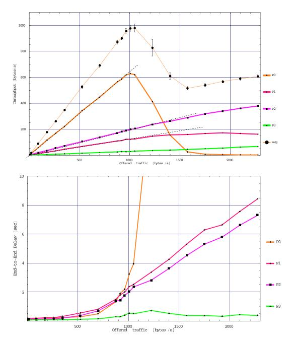
Figure 10.10 Simulated performance for time instance  $t_1$ . Confidence control is only applied to the cumulative throughput plot.
