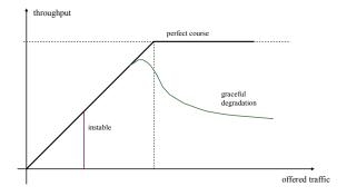
Figure 9.11 Illustration of possible throughput progress versus offered traffic.
