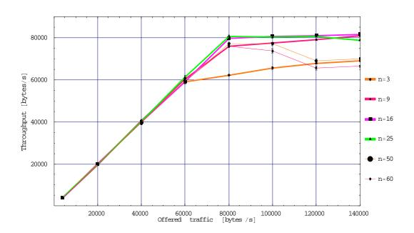
Figure 9.12 Estimated throughput using multiple priority levels. The priority distribution is {P0,P1,P2,P3}={0.4,0.3,0.2,0.1}. The legend expresses the network size as number of nodes. Radio version: 1Mbps. (simFeb2a).
