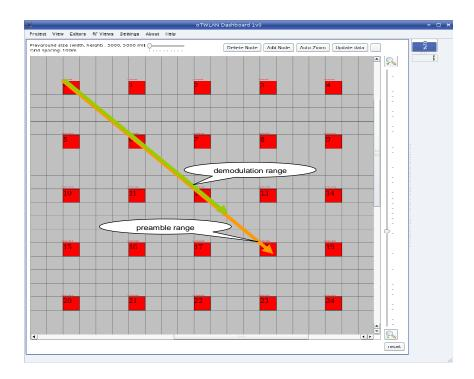
Figure 10.12 The playground layout with grid spacing 100 meters. The node positions are the upper left corners of the red boxes. The arrows indicate the preamble range and the demodulation range for node 0 when it sends at -10 dBm.
