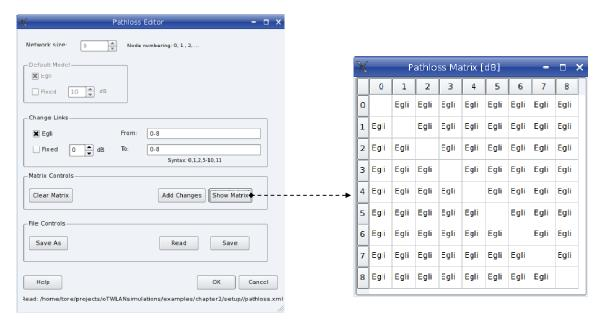
Figure 2.4 The pathloss editor (class GUI\_PathlossEditor) facilitates setting of a pathloss model on a per link basis.
