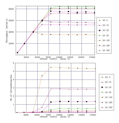
Figure 9.5 Throughput as 90% confidence intervals (top picture) for the 1Mbps radio version.
