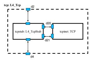
Figure 4.6 The coupled model L4\_Tcp contains the atomic module TCP which is implemented by the INET-project [1]. The atomic module L4\_TcpStub is designed to be a wrapper between the INET software and the oTWLAN software.
