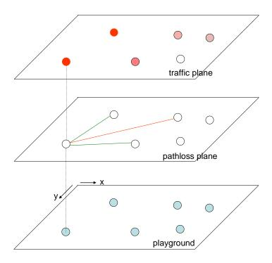
Figure 5.1 Modelling the network environment. These layers must be configured in sequence, starting at the bottom layer. The nodes are assigned unique identifiers within the playground plane and these identifiers are used within the other two planes.
