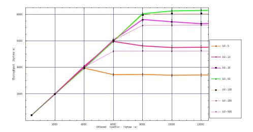
Figure 9.2 Throughput (90% confidence intervals) as function of the offered traffic. Only priority P3 traffic is used. Radio version: 100kbp (simDec11a).
