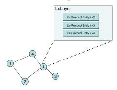
Figure 6.8 The internal data structure of the LLC Layer module. Node i creates three separate objects of the class L2\_LlcProtocol; one for each of its three neighbours in the topology shown.
