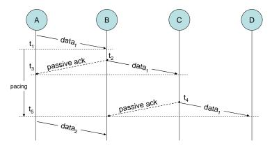
Figure 3.6 Time-sequence diagram for packet forwarding. Related data packets are tagged with the same number (GId).
