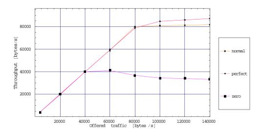
Figure 9.10 Simulated network throughput using multiple priority levels. The priority distribution is {P0,P1,P2,P3}={0.4,0.3,0.2,0.1}. Radio version 1Mbps.
