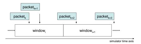
Figure 5.12 Rate probes collect samples over a time window.
