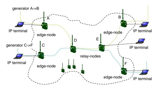
Figure 3.1 An example network with two traffic generators representing the terminal applications.
