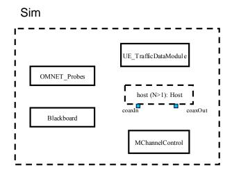
Figure 4.2 The top level of the model is a coupled model containing both atomic and coupled models.
