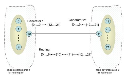
Figure 10.4 The scenario is divided into three radio coverage areas. Two regions contain 11 nodes and one region contains the two nodes {10,11}.
