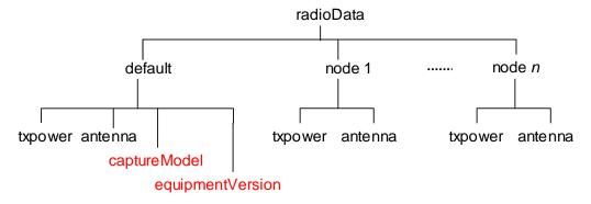
Figure 5.10 The structure of the radio data.
