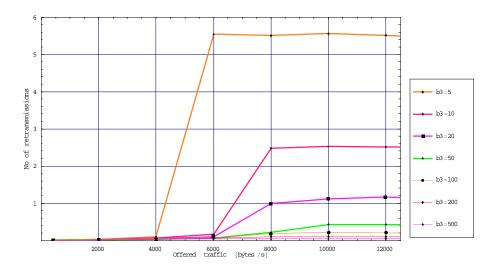
Figure 9.3 The course of the number of retransmission with increasing load level for radio version 100kbps. Estimation is done without confidence control (simDec11a).
