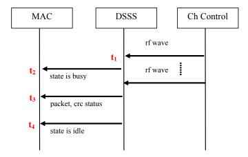
Figure 6.11 Sequence diagram for incoming packet over the air interface
