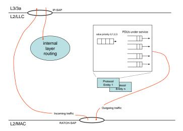
Figure 3.10 The queue structure within the LLC layer. Each LLC entity can store only one (1) fresh PDU per priority. PDUs under service are PDUs ready to be sent (acknowledgments or retransmissions), or PDUs awaiting acknowledgment.
