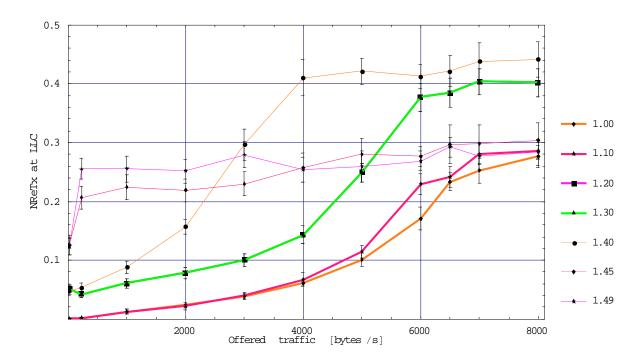
Figure B.2 Average number of retransmissions at the LLC layer retransmission versus offered traffic. The legend expresses the link cost limit applied. The plot for link cost 1.20 and 1.30 are identical.
