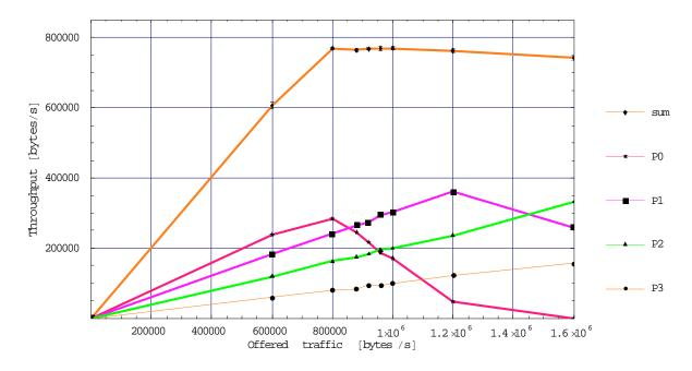
Figure 9.8 Throughput versus offered traffic. No confidence control is used for the plots showing throughput per priority. Radio version: 10Mbps (simNov26b).
