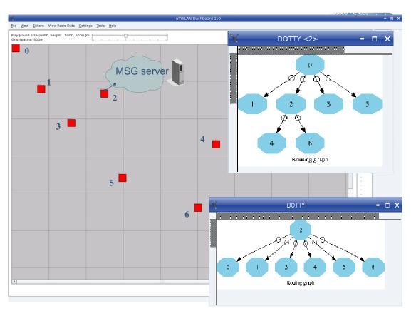
Figure 5.9 The routing graph for node 0 and node 2.
