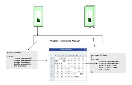
Figure 4.9 The MChannelControl module models the physical transmission medium.
