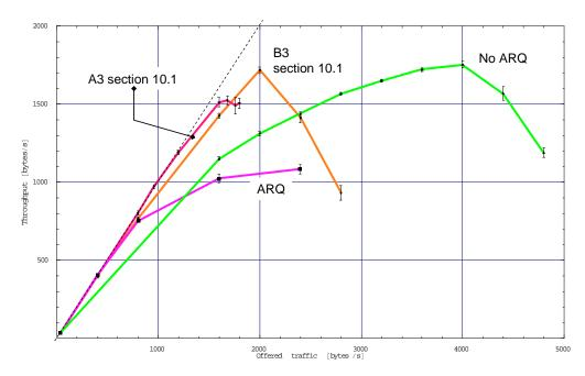
Figure 10.5 Simulated throughput versus offered traffic using a two-way traffic pattern between the two 10-node groups (simFeb23a).
