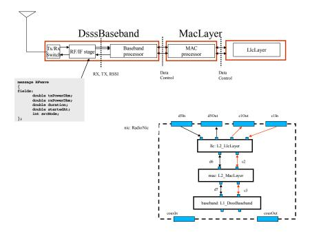
Figure 4.7 The topmost figure depicts an RF wave that arrives at the receiver and shows the internal structure of a radio card. Functional split of the RadioNic into atomic modules is shown in the bottom figure. Incoming RF waves arrive at the coaxIn port.
