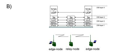
Figure 3.2 Layered models. Figure a) shows the protocol stack for a real system while b) shows the stack implemented in the simulator. The 3b layer protocol carries layer 3 information which is not needed by relay nodes but must be signalled end-to-end.
