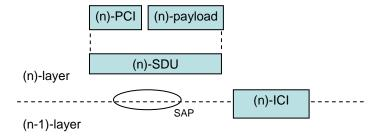
Figure 6.1 General principles for encapsulation and interface control.
