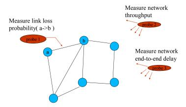
Figure 2.13 Probes are the objects that collect and process samples from probability distributions.
