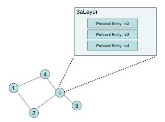
Figure 6.7 The internal data structure of the L3\_3aLayer module. Node i creates three separate objects of the class L3\_3aPDP; one for each of its three neighbours in the topology shown.
