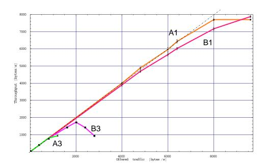
Figure 10.2 Simulated throughput versus offered traffic for the cases A1, A3, B1 and B3. 90% confidence intervals (simFeb17d).
