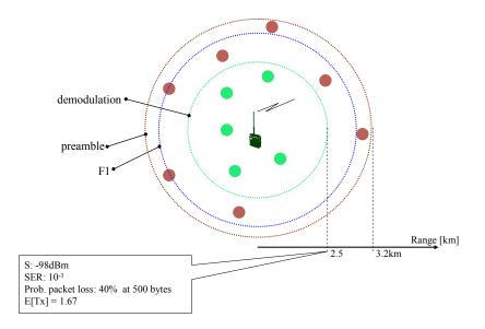
Figure 2.6 Radio frame coverage prediction when sending at 10 dBm (10 mW).
