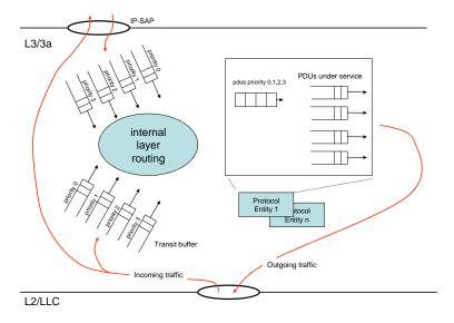
Figure 3.7 The queue structure within 3a layer. Queuing is done on a per PDU basis according to its type and priority level.
