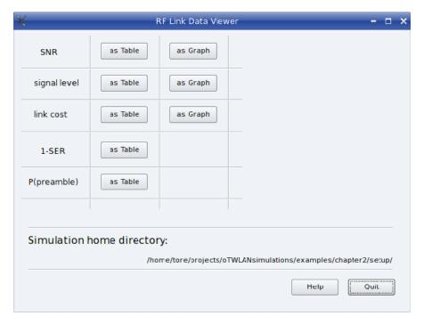
Figure 2.7 The "RF Link Data Viewer" (class GUI\_RfLinkViews) provides widgets to assist the user in the radio planning phase. The widget is activated from the menu "View Radio Data"->"Rf Link Data".
