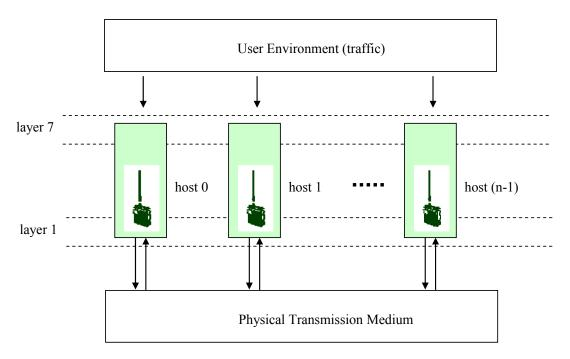
Figure 4.1 The basic structure of the oTWLAN model.
