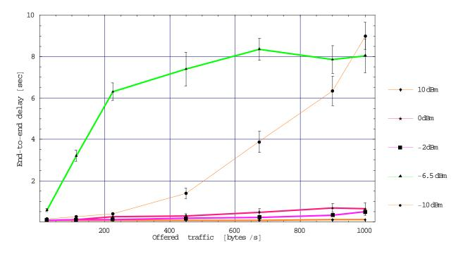
Figure 10.14 End-to-End delay versus offered traffic.
