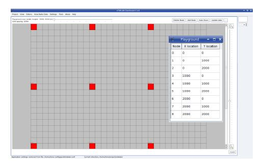
Figure 2.3 The oTWLAN dashboard (class GUI\_MainWindow) provides a set of functions to set up simulation scenarios, run simulations and analyse results.
