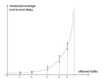
Figure 2.11 A simulation session where the objective is to measure the end-to-end delay as function of the offered traffic. We want to have control of the quality of the estimates and present the measurements as confidence intervals.
