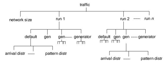
*Figure 5.5* The network traffic represented as a graph with the top node <traffic>.
