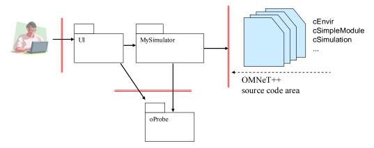
Figure 8.1 The analysis model for the oTWLAN project. The three most important interfaces to the external environment are shown as red lines. The solid arrows should be read as "depends on" (e.g., the UI-package depends on the oProbe-package).
