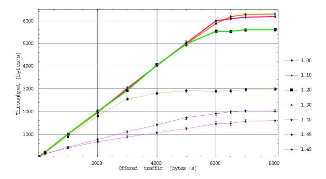
Figure B.1 Throughput versus offered traffic. The legend expresses the link cost limit applied.
