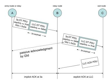
Figure 3.3 The 3a layer protocol utilises the broadcast feature of radio communications by using passive acknowledgement on the intermediate hops and explicit acknowledgement on the last hop.
