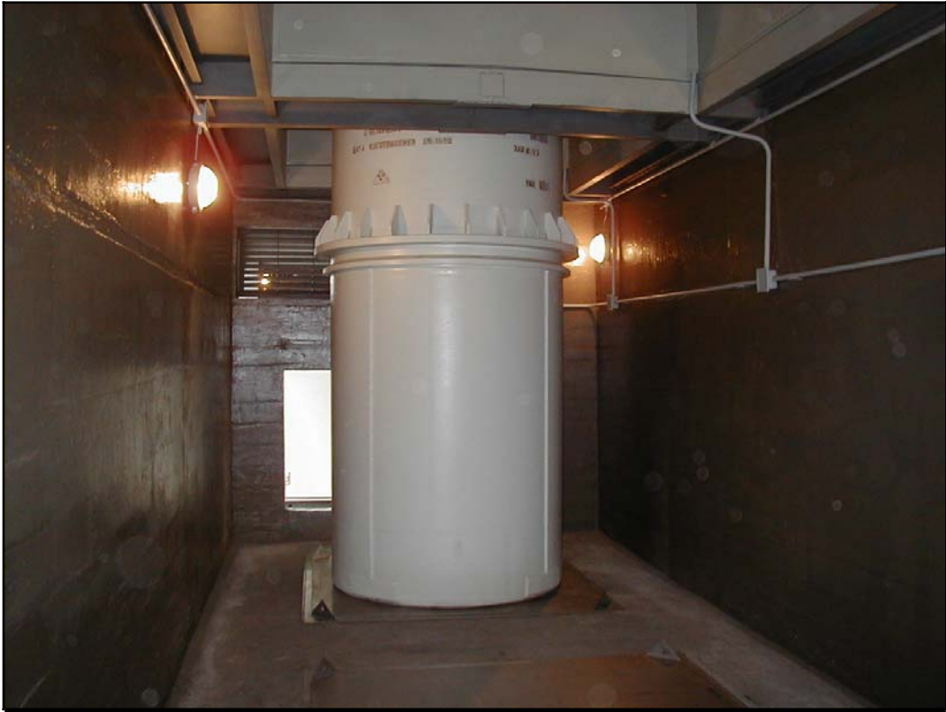
Fig. 1. The TUK-108 Prototype Container in one of the 19 storage cells during cold-testing of the Transshipment/Interim Storage Facility, June 2003.
