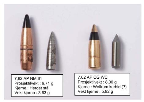
Figure 3.1: The projectiles and cores that are studied in this report.
