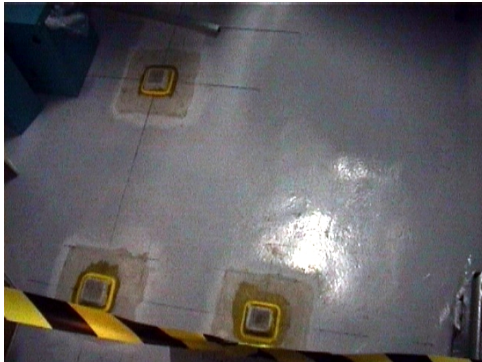
Figure 3.21 Hats on the instrument room floor onto which the jig for rotation measurements was mounted
