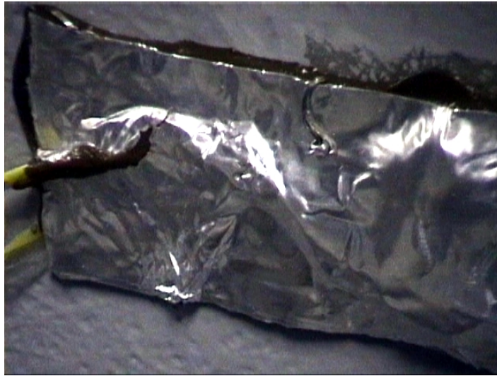
Figure 2.4 Strain gauge with ABM 75 aluminum shield. Notice the ground wire pierced through the foil
