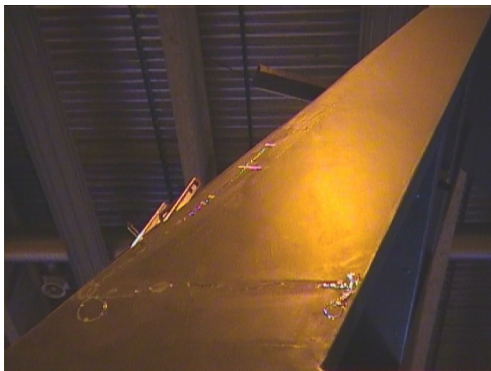
Figure 3.25 Fiber Bragg grating installation on the port side mast
