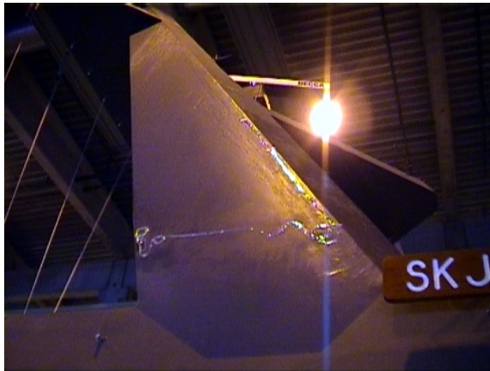
Figure 3.24 Fiber Bragg grating installation on the starboard side mast
