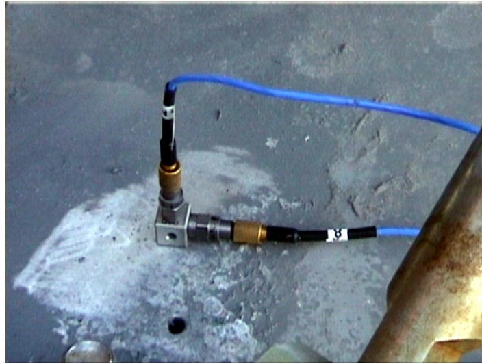
Figure 2.5 Two accelerometers mounted on a precision cube glued to the radar fundament using cyanoacrylate glue
