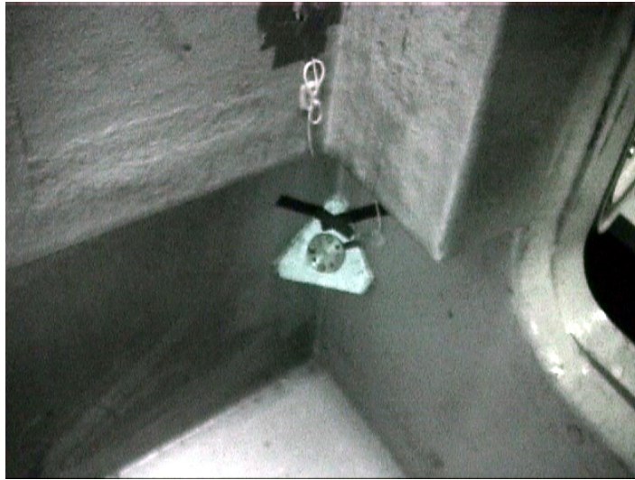
Figure 3.12 Pressure sensor P5 was mounted in a Styrofoam holder somewhat above the lower corner on the forward port side in the lift fan room
