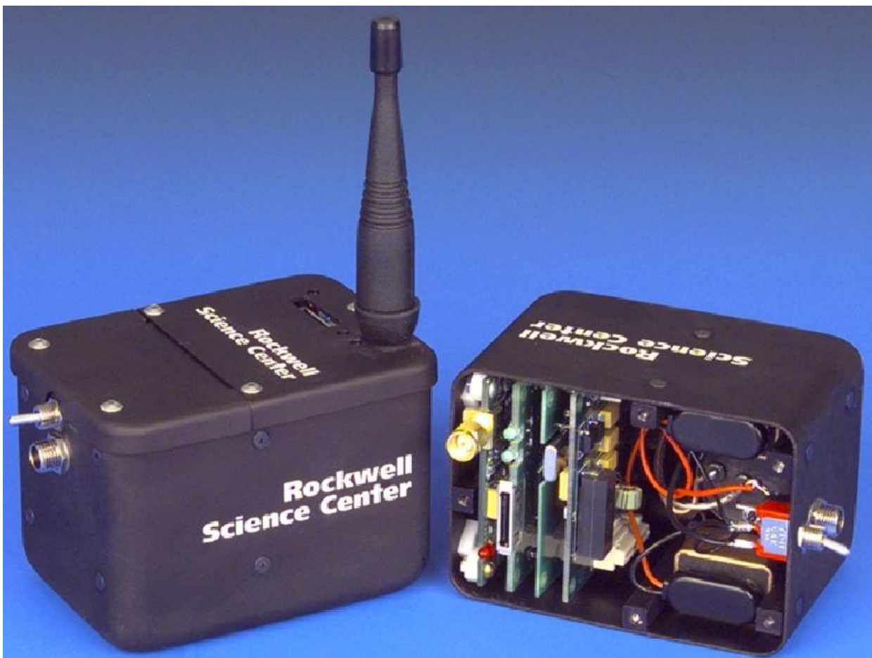
Figur 4.8 AWAIRS I prototyp sensornode (Kilde: www.rockwellscientific.com )
