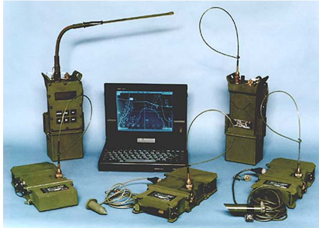
Figur 3.15 Komponenter i REMBASS-II systemet (Kilde: www.army-technology.com/contractors/navigation/1-3/index.html )
