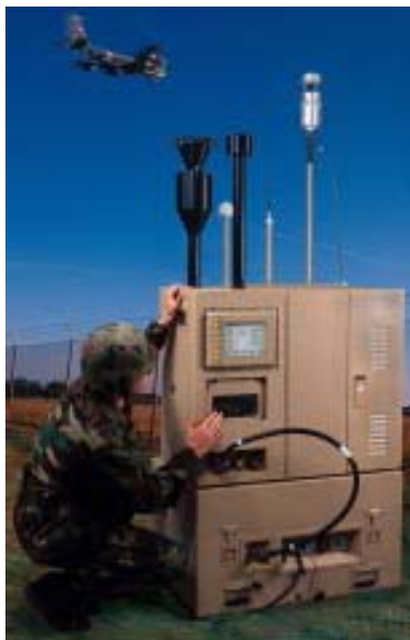
Figur 3.3 Joint Biological Point Detection System (Kilde: www.braddocksmithgroup.com/pdf/CONTAMINATION_AVOIDANCE.pdf )
