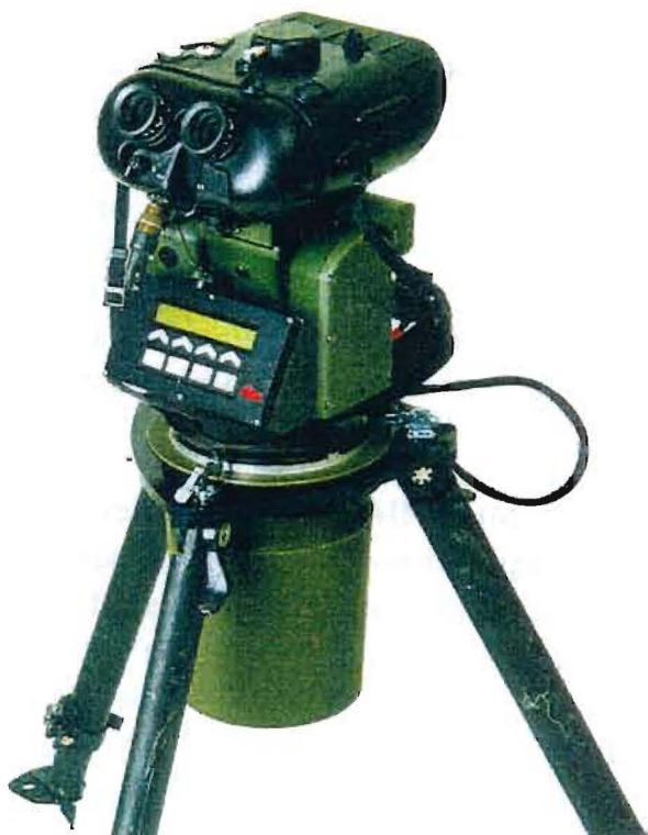
Figure 2.1 Forward Observer Instrument - Functional Model Top: Main Module (LP10), Middle: Goniometer (SG12), Bottom: North-Finder
