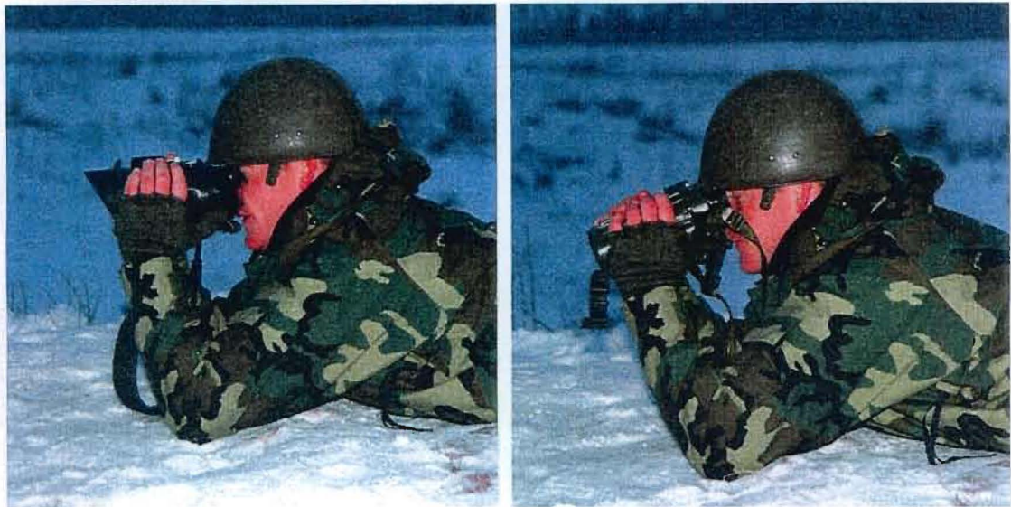
Figure 5.1 Ergonomics: Tilted and straight eyepieces with helmet. Left: The functional model with tilted eyepieces. Right: Laser range-finder (LE7) with straight eyepieces. Notice the aiming direction in the right image. The operator has difficulties when trying to aim horizontally due to conflict with the helmet.
