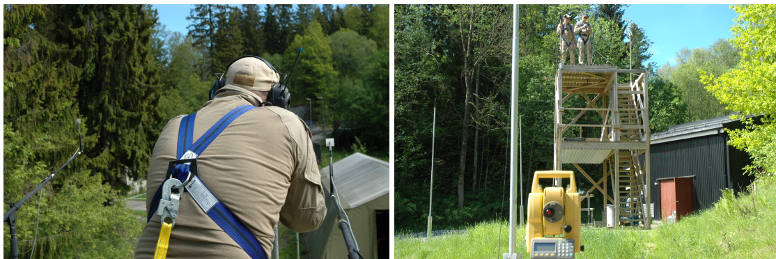
Figure 2.1 Placement of the sensors. The reflectors seen on the sensors are removed before measurement, and is used for measurement of sensor positions with Topcon GPT 3107NW.
