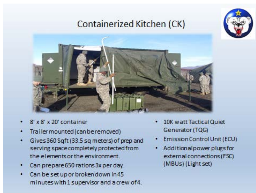
Figur 4.10 Konteinerbasert feltkjøkken (Scott 2014)
