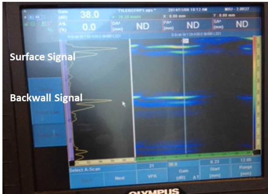
Figure 9.6: Signals from the surface and back wall of a panel.
