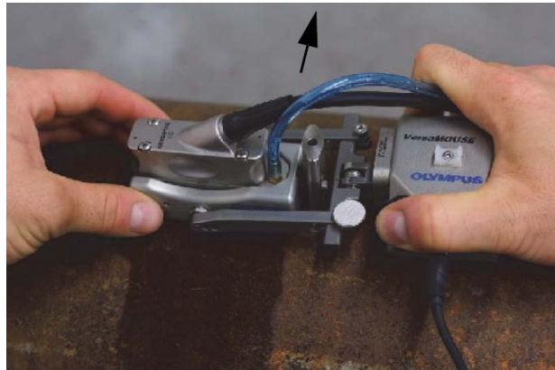
Figure 9.7: Performing a C-scan with VersaMOUSE.
