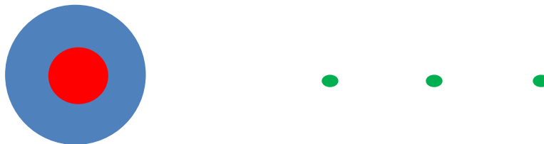
Figure 7.1 Illustration of DSTL-experiment: Charge in red, damping material in blue, gauges in green.
