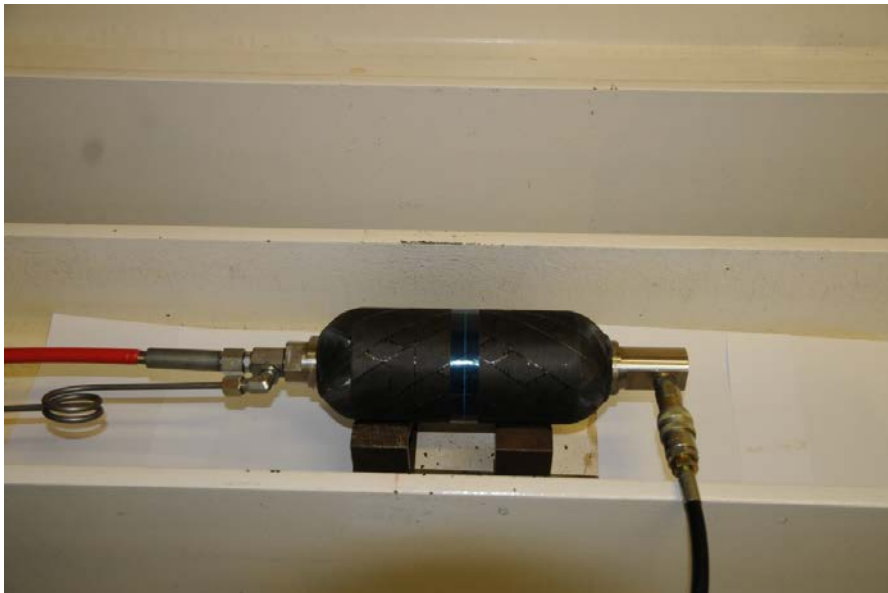
Figure 2.1 Mounting of the pressure vessel in the burst test chamber.
