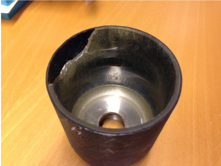
Figure 3.24 Pressure vessel CP-10, which is cut open. The liner thickness is approximately 3 mm.
