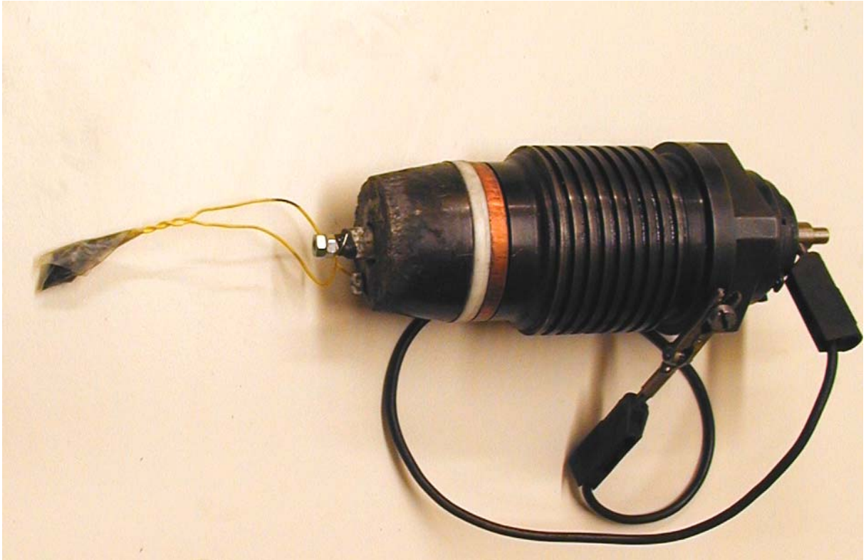
Figure 2.1 Ignition part of the CV, showing the squib surrounded by a plastic bag with the Black Powder.
