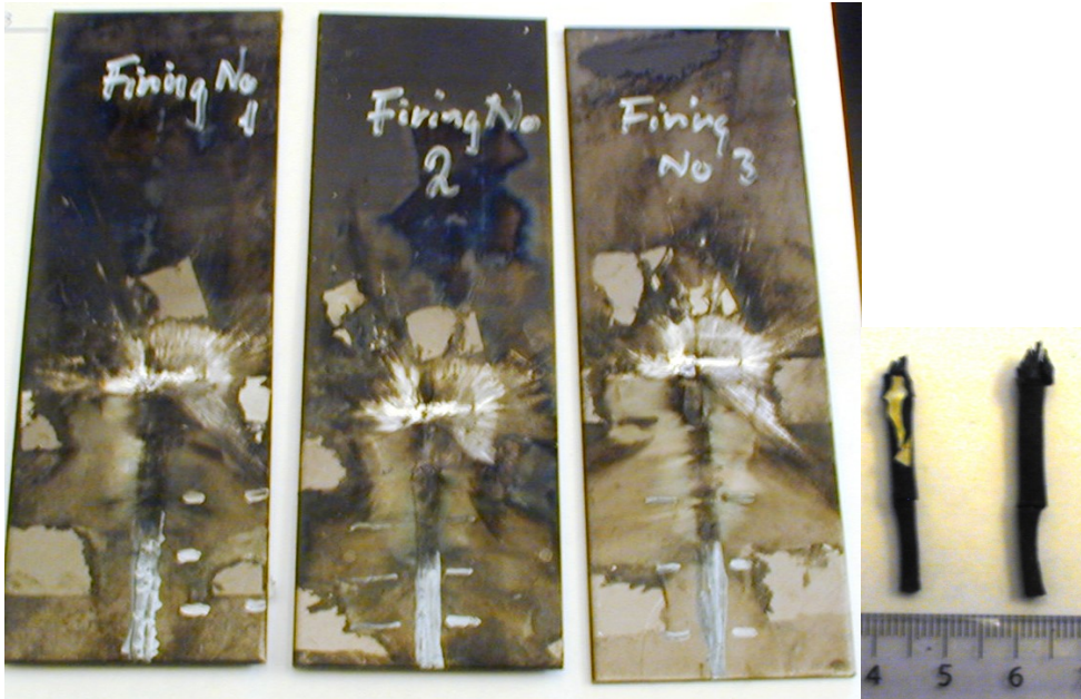
Figure 3.9 Picture of the witness plates from the three firings of cylindrical charges. To the right is a picture of the recovered rests of the test items No 1 and No 3.
