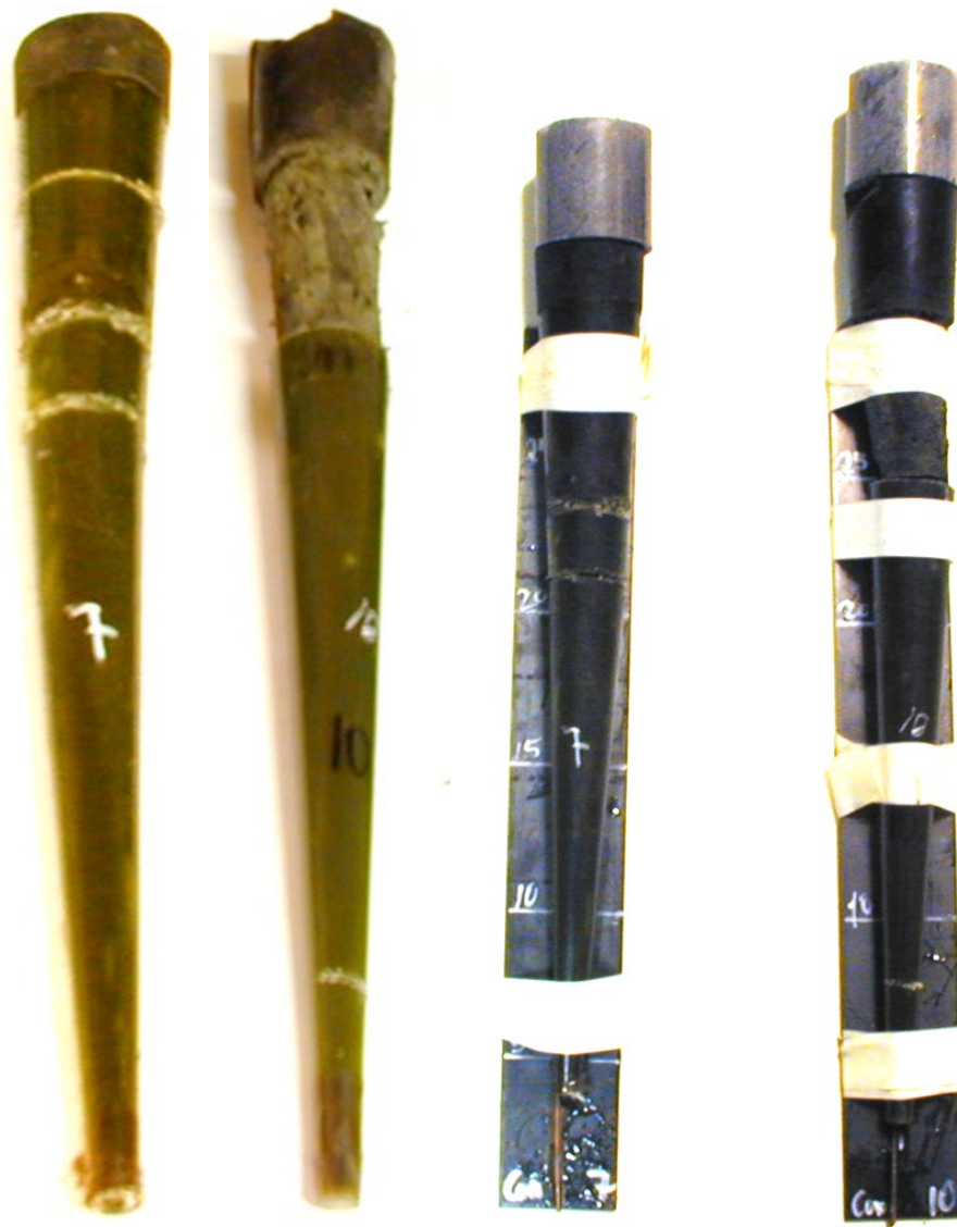
Figure 2.3 Conical charges No 7 and No 10 in the mould to the left, to the right after being placed on the witness plates and added boosters.
