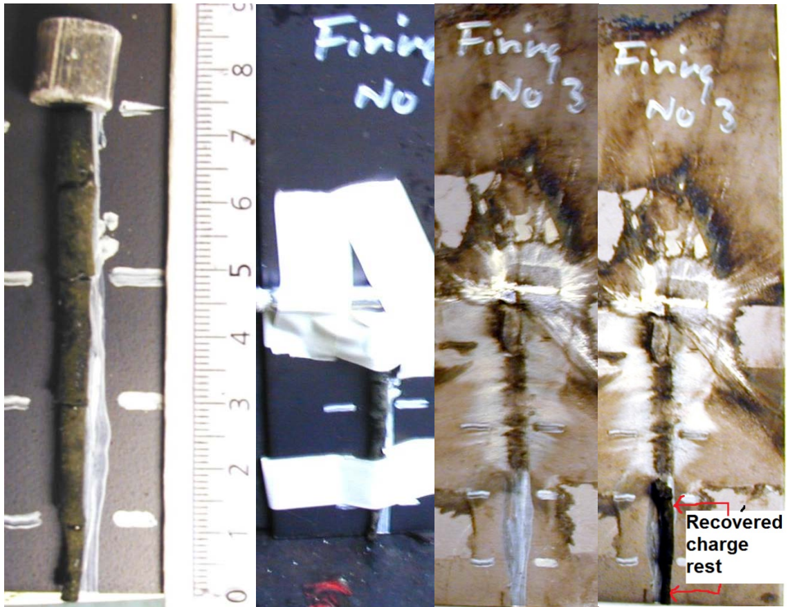
Figure 3.8 Pictures of test item No 3 before firing (to the left), the setup, and to the right the witness plate with and without the recovered part of the test item after firing.
