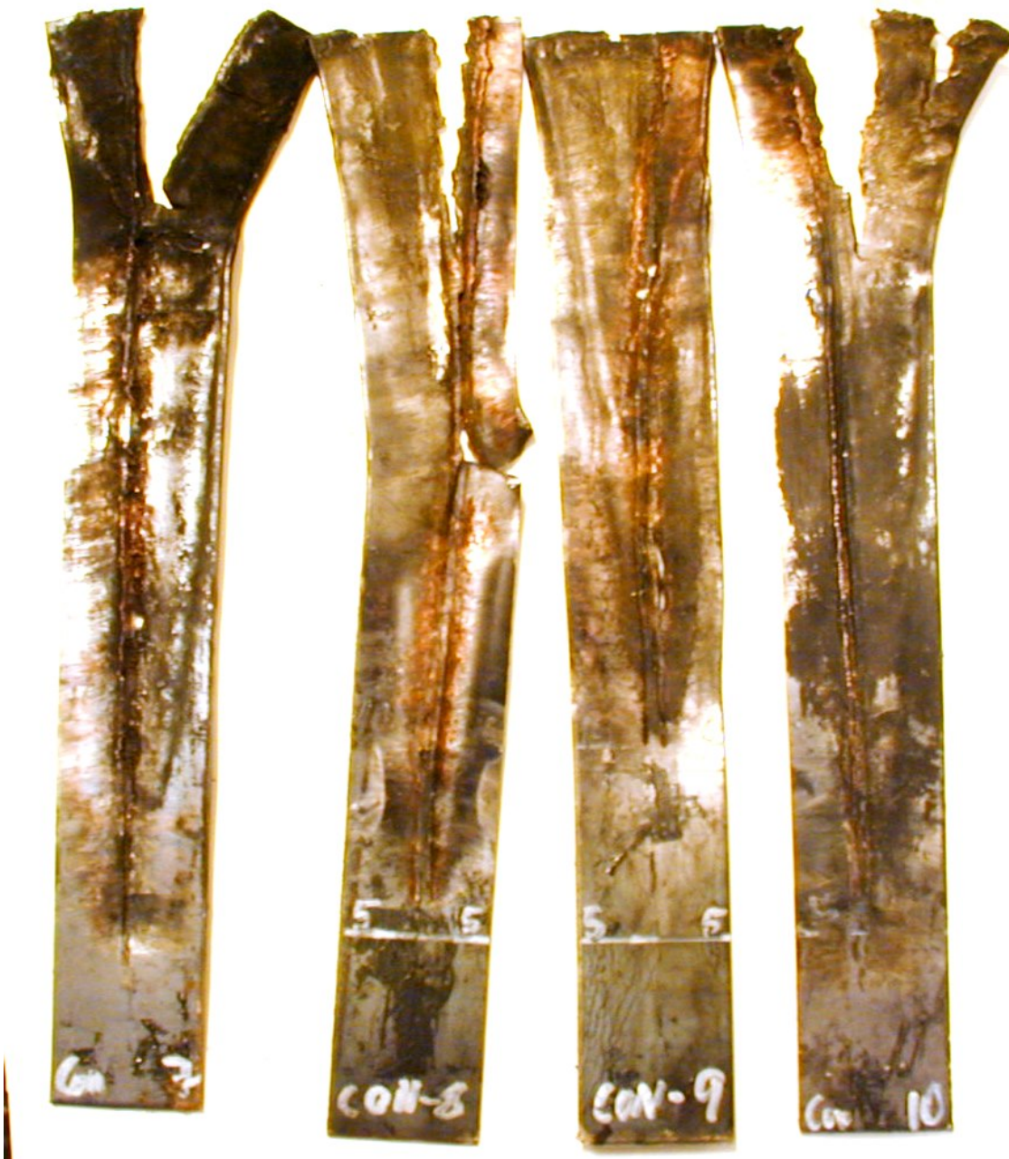
Figure 3.5 Picture of the witness plates from the firings of the 4 conical test items.
