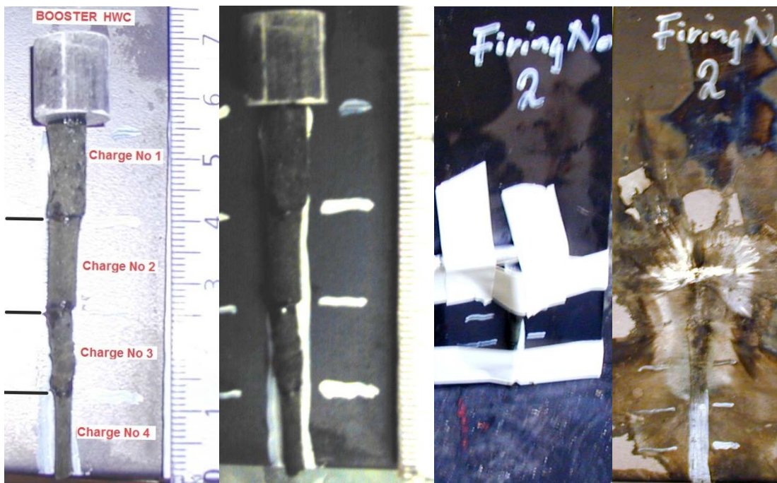
Figure 3.7 Pictures of test item No 2 before firing (to the left), the setup, and to the right the witness plate after firing.
