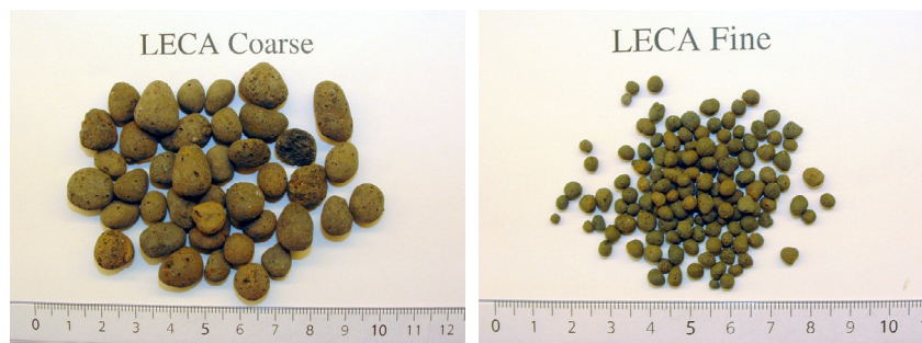
Figure 3.2 Coarse and fine LECA used in the damping experiments.
