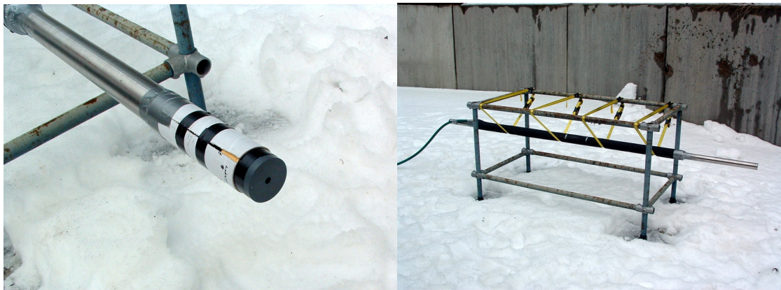
Figure 4.1 The experimental set-up, showing the cardboard tube containing the explosive charge and the damping material fitted onto the steel bar.
