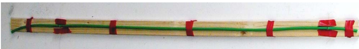
Figure 3.2 Picture of the detonating cord used to test registration equipment and cabling.
