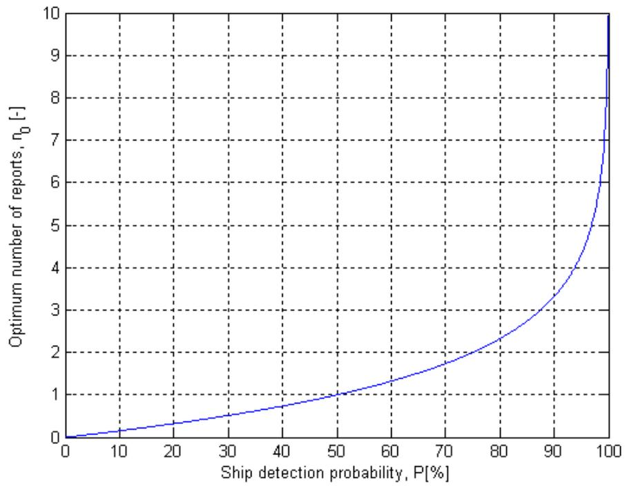
Figure 5.43 Optimum number of reports as a function of ship detection probability.
