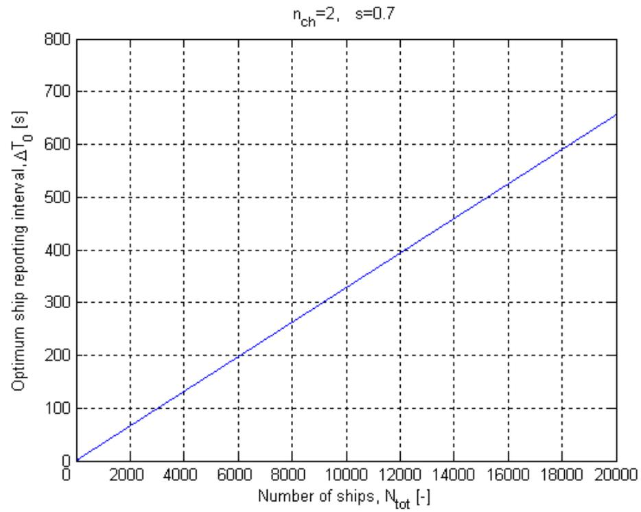
Figure 5.44 Optimum ship reporting interval as a function of number of ships.
