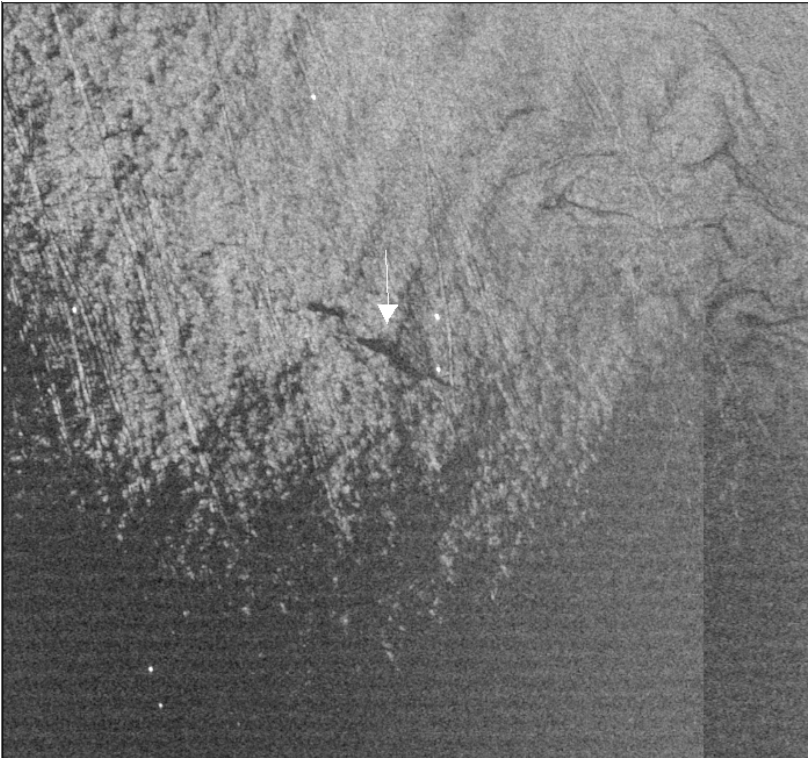
Figure 1.2 Section of an ENVISAT ASAR Wide Swath Mode (WSM) image (3 August 2003). Oil spill (indicated by arrow) surrounded by low wind look-alikes. The oil spill has been classified as oil by a German surveillance aircraft. © ESA/KSAT 2003.
