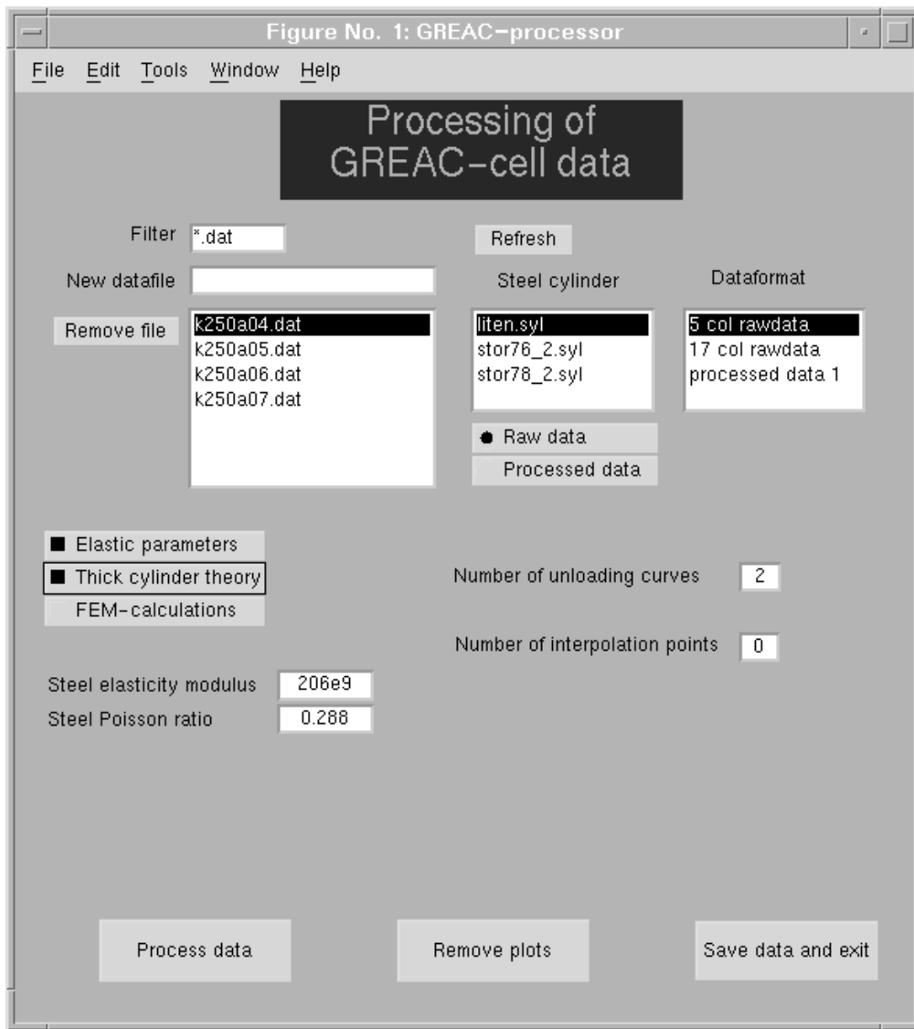
Figure 5.2 The menu based program for processing GREAC-cell data.
