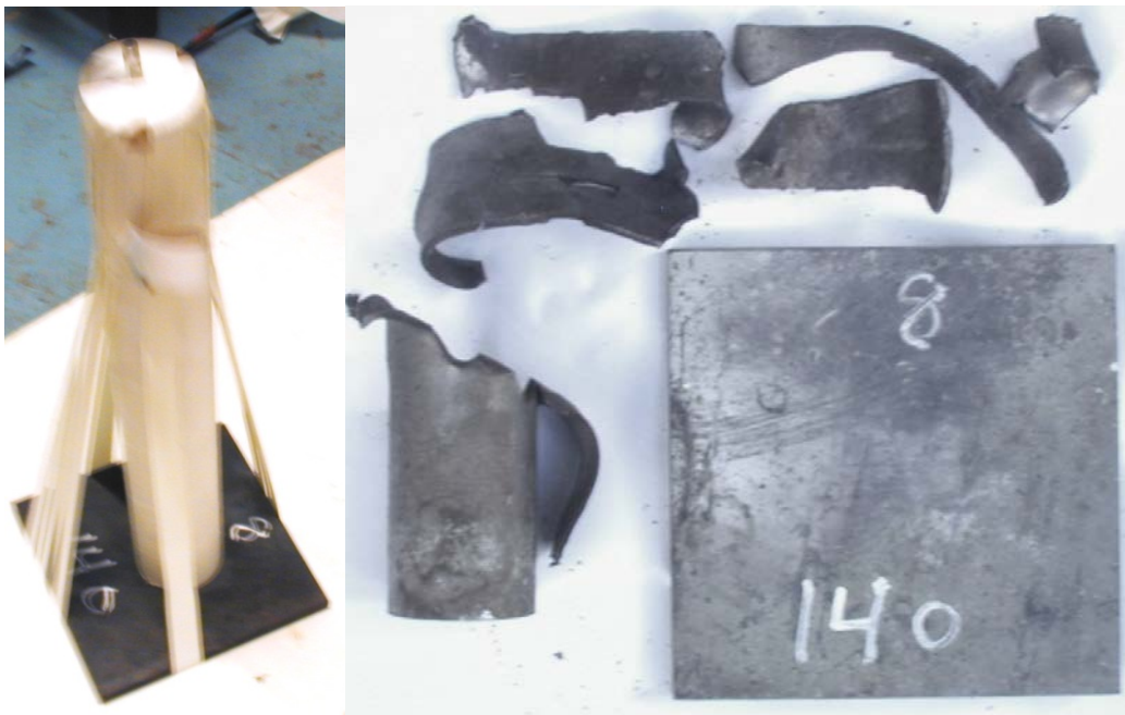
Figure 3.8 Firing No 8, tube No 10, barrier thickness 140 cards. Response: No reaction. The weight of the recovered tube remnant is 694 g.
