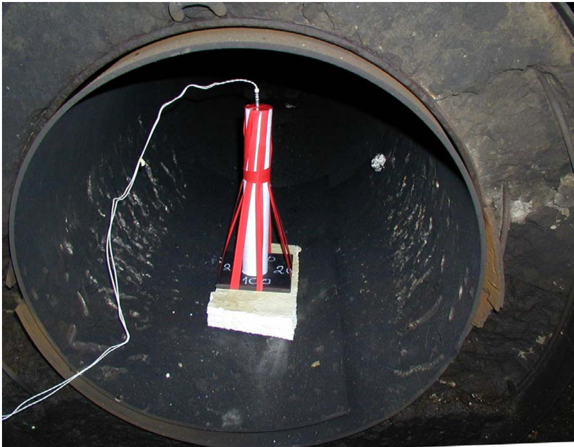
Figure 2.12 The picture shows the test setup for firing of the gap test tubes.
