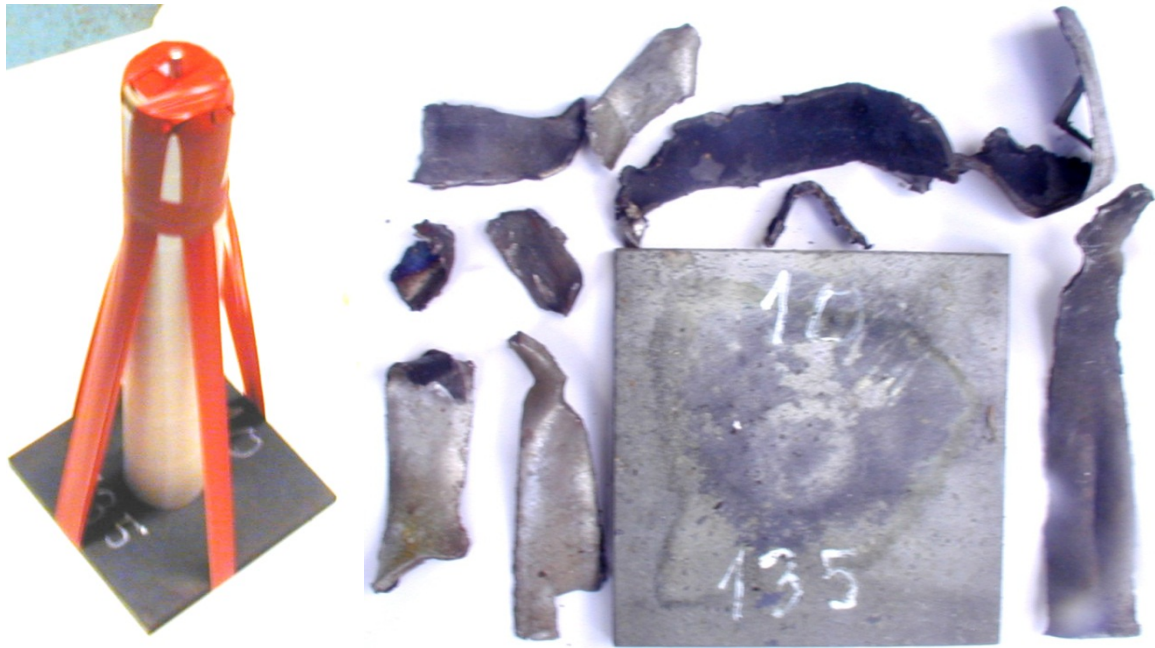
Figure 3.10 Firing No 10, tube No 21. Barrier thickness: 135 cards. Response: No reaction. The weight of the recovered tube remnant is 633 g.
