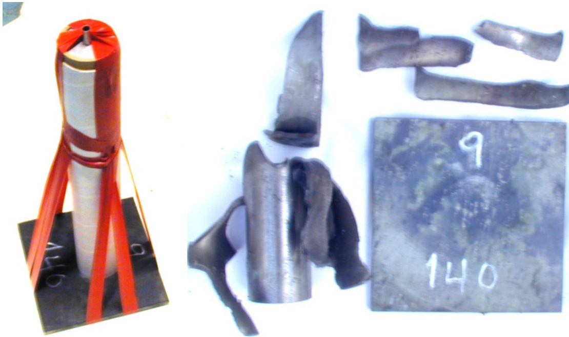
Figure 3.9 Firing No 9, tube No 11, barrier thickness 140 cards. Response: No reaction. The weight of the recovered tube remnant is 831.74 g.
