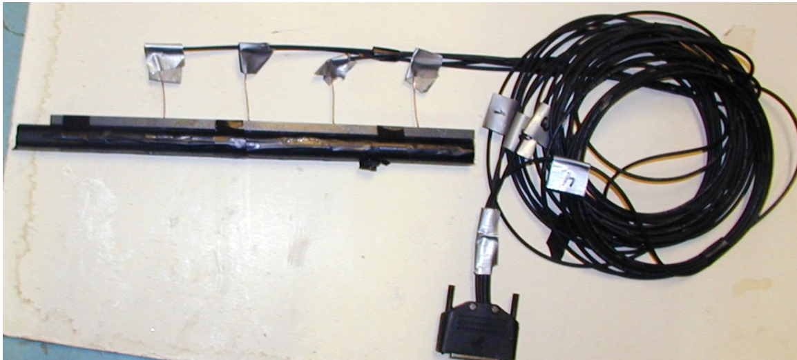
Figure 3.8 Picture of the test item after the ionization pins were put into the charge.
