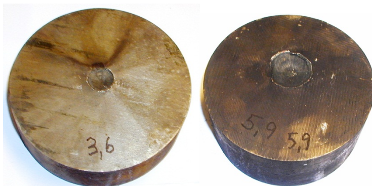
Figure 3.14 Pictures of the Dent Plates after the two firings with HWC.
