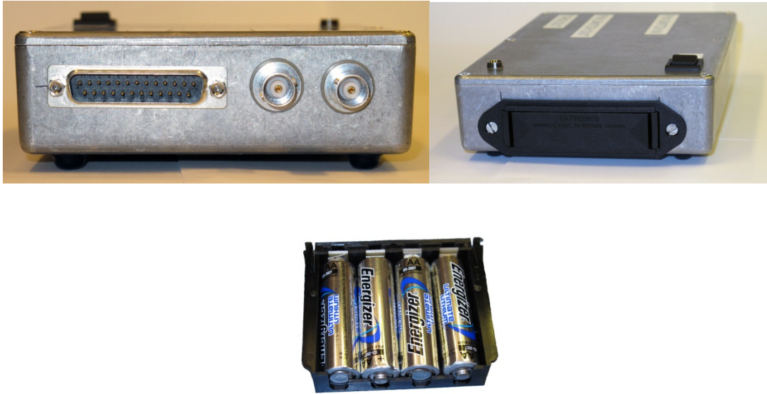
Figure 2.3 Picture of the end of the switch box and the power supply unit.
