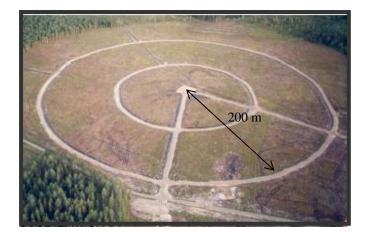
*Figure 6.* The region used for biological field trials located near the Swedish Defence Research Agency FOI, Umeå. The biological detection equipment is located in the center of the field. The release of the biological simulants takes place at a 100 or 200 m distance in radius from the equipment.
