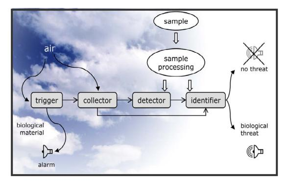
*Figure 3.* An optimal biological detection warning system and the following necessary identification process of airborne biological agents.
