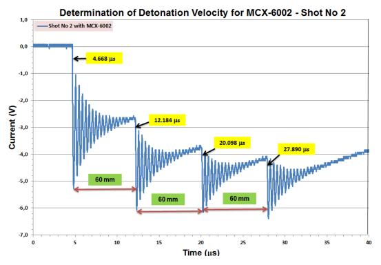
*Figure 3.12 The figure shows the arrival time of the detonation front for each pin and the distance between pins.*
