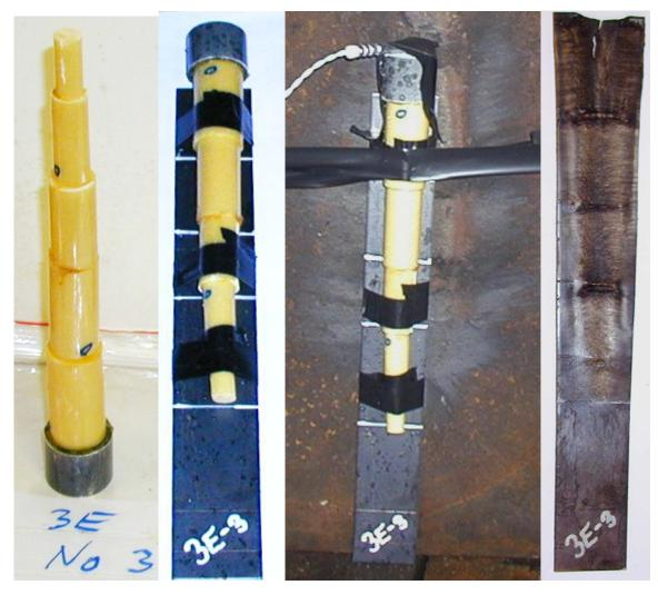
*Figure 3.3* Different pictures: from left the test item after being glued together, next after the test item had been assembled on the witness plate, setup for firing and to the right the witness plate after firing.
