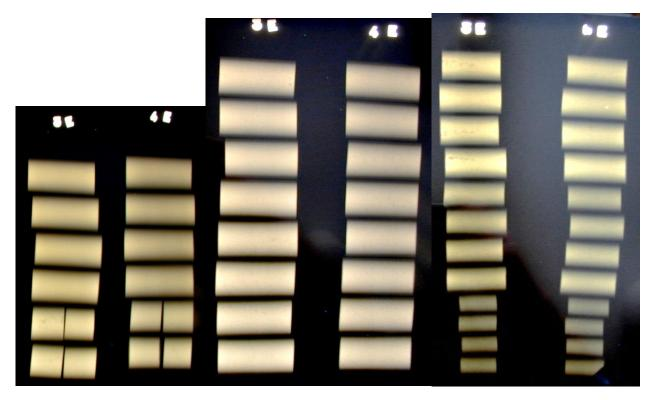
Figure 2.7 Pictures of X-ray films of the items in Figure 2.6. Charges marked with 3E contain composition MCX-6002 and 4E contain composition MCX-8001.
