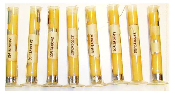
Figure 2.1 Filled moulds, 4 with MCX-6002 (left) and 4 with MCX-8001 (right) compositions after the melt had solidified.
