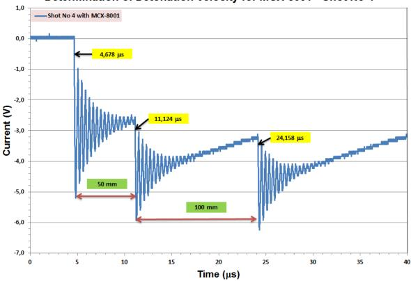
Determination of Detonation Velocity for MCX-8001 - Shot No 4
