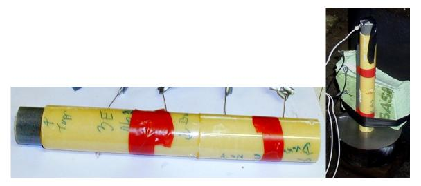
*Figure 3.11 Left picture shows the charge after the ionization pins had been positioned. Right picture shows the charge setup for firing.*
