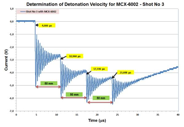
*Figure 3.14 The figure shows the arrival time of the detonation front for each pin and the distance between pins.*
