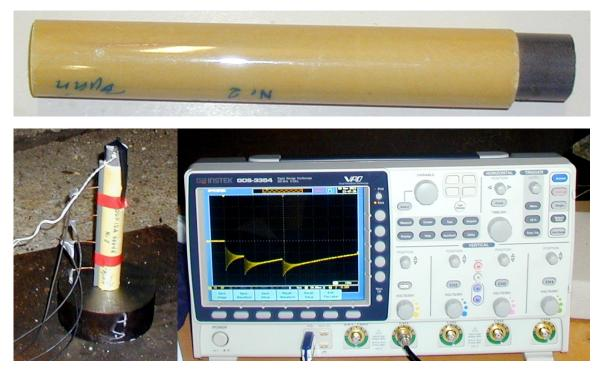
Figure 3.20 The first picture is of the test item; second left test setup for firing and on right a picture of the used scope with the obtained registration.
