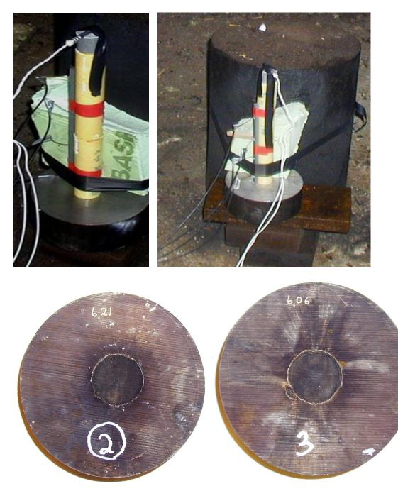
Figure 3.24 The Figure shows the setup and the Dent plates after firing for the two tested charges containing the MCX 6002 composition.
