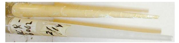
Figure 2.8 Picture of the MCX-6002 CH 6080/13 conical charge cast No 7/14.
