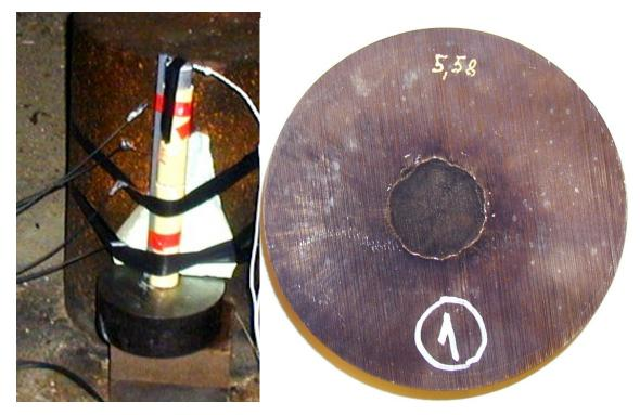
Figure 3.25 Left picture shows the test setup and the right picture the Dent plate after the firing.
