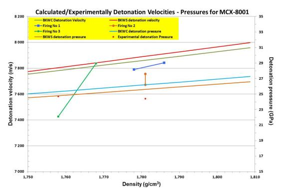
Figure 3.28 Calculated and measured detonation velocities and detonation pressures for MCX-8001 as function of density.
