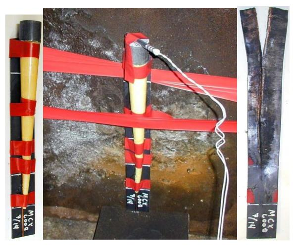
*Figure 3.4* The figure shows from left; the test item after assembled, test setup for firing and to the right the witness plate.
