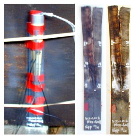
Figure 3.6 The figure shows test setup and witness plate for firing of conical charge cast 12/14 containing MCX-6002 CH 6080/13 composition.
