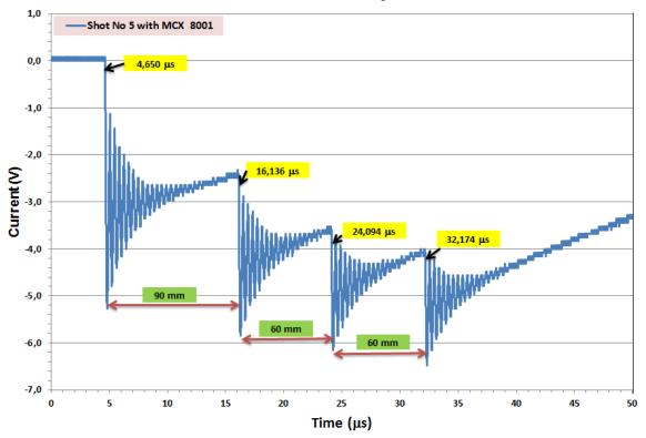
Determination of Detonation Velocity for MCX 8001- Shot No 5
