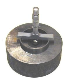
Figure 2.14 Picture of the tool used to measure the Dent depth.
