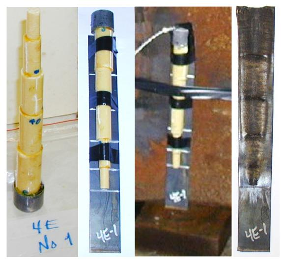
*Figure 3.8* Different pictures: from left the test item after being glued together, next after the test item been assembled on the witness plate, setup for firing and to the right the witness plate after firing.
