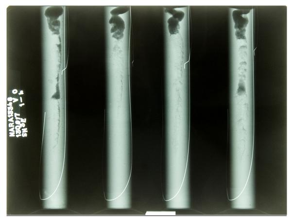
*Figure 2.2* The figure shows the X-ray picture of the four tubes filled with MCX-6002 composition.
