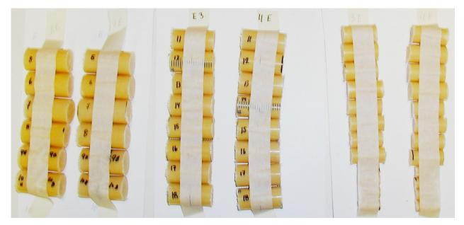
*Figure 2.6 Pictures of the smaller charges casted for critical diameter and mechanical testing. Charges marked with 3E contain composition MCX-6002 and 4E contain composition MCX-8001.*
